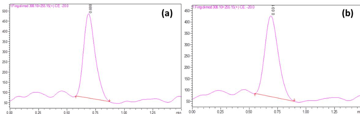
Figure 2: (a) standard chromatogram and (b) sample chromatogram of Fingolimod.
