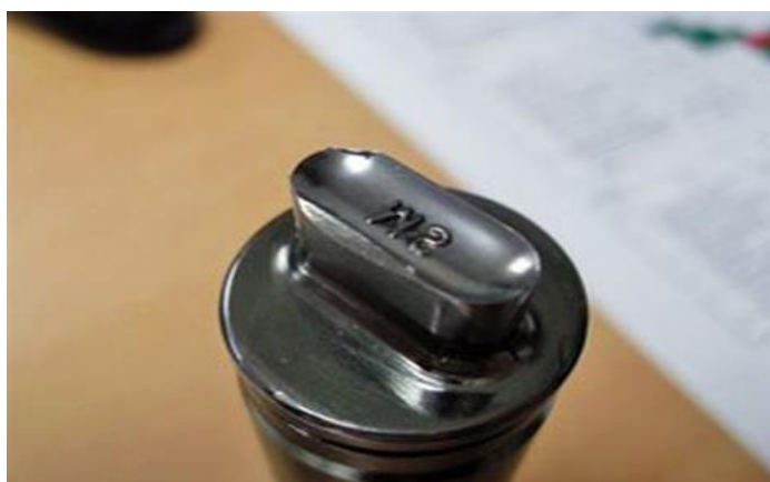
Figure 1: Damage to punch-tip land area can be caused by poor handling.
