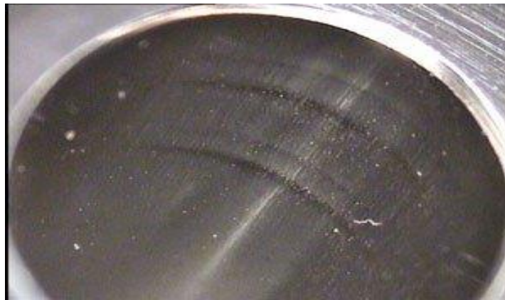
Figure 4: Die-bore wear appears as a double ring.
