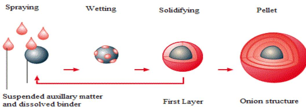
Fig.7.Principle of the Suspension and Solution Layering Process.
