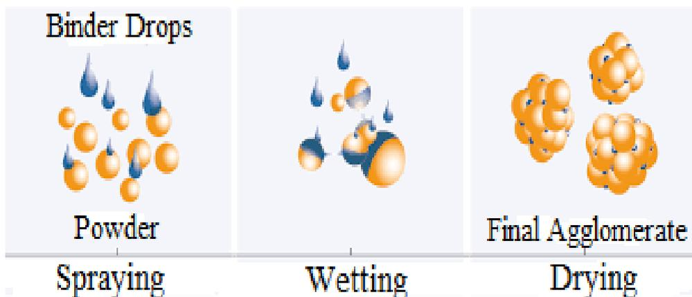
**Fig.3. Process principal of drying solids.**
