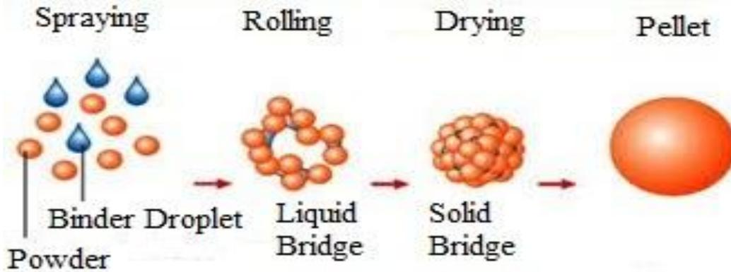
Fig.5. Process Principle of Direct Pelletizing.
