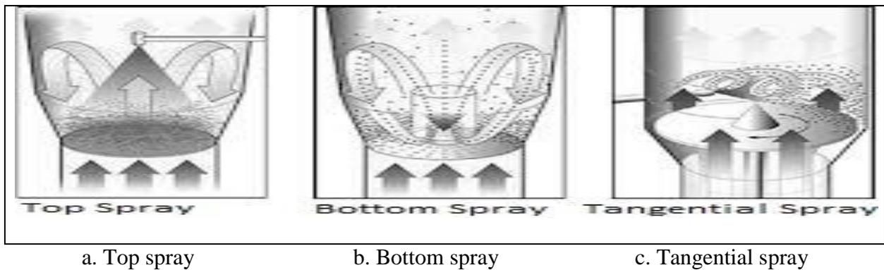
**Fig.2. a. Top spray, b. Bottom spray, c. Tangential spray.**
