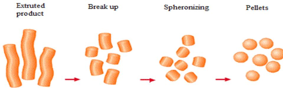
**Fig.9. Principle of the Extruded Product Spheronizing Process.**
