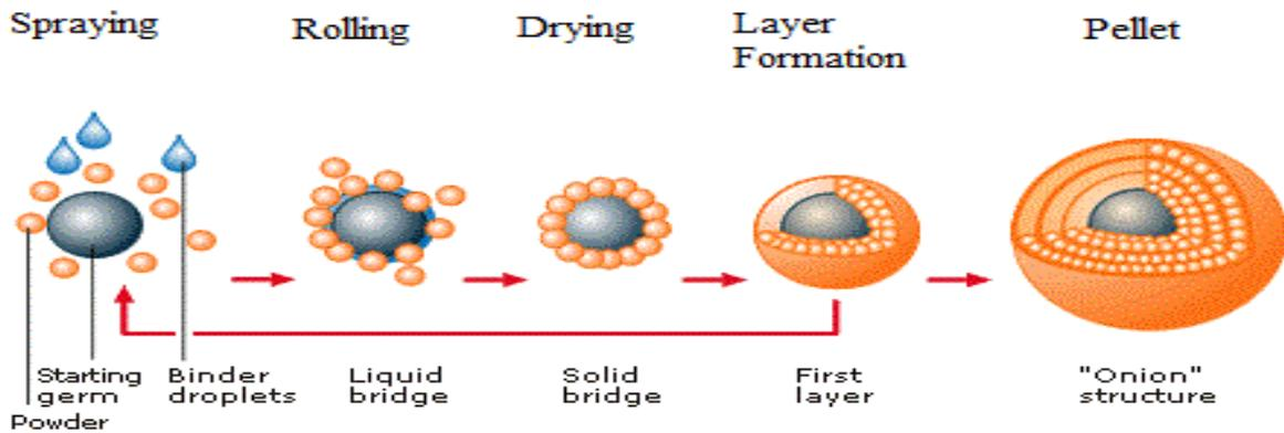
Fig.6. Principle of the Powder Layering Process.
