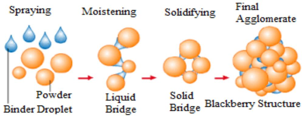
Fig.4. Process Principle of Spray Agglomeration.
