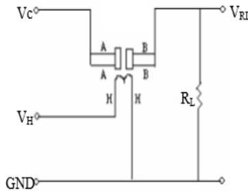
**Fig. 2: Alcohol Sensor.**
