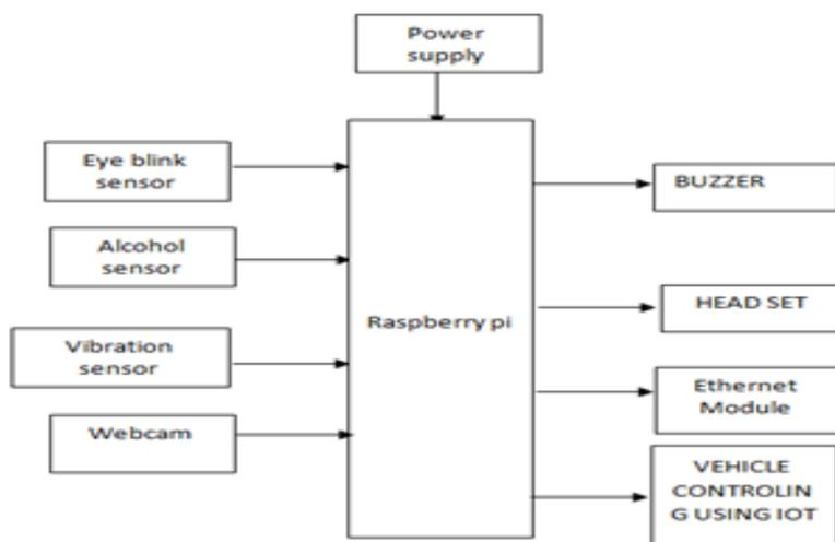
**Figure 1. Vehicle Accident Detection System.**
