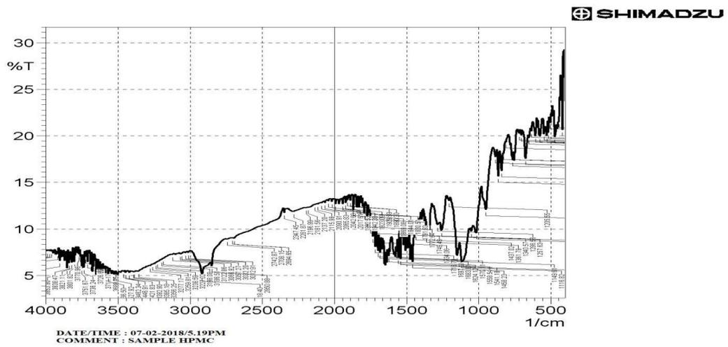
FIG:3 FT-IR of HPMC K 100M.
