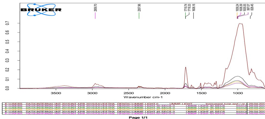
**Figure-2:** Graph representing the FTIR spectra of an uncured and cured light cure resin at 30,35,40,45 and 50 seconds using ATR-FTIR.
