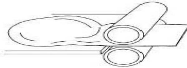
**Fig :7 Apparatus used in Rolling Method of preparing oral wafers.**
