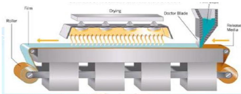
**Fig 5: Industrial manufacturing of oral wafers by Solvent casting method.**
