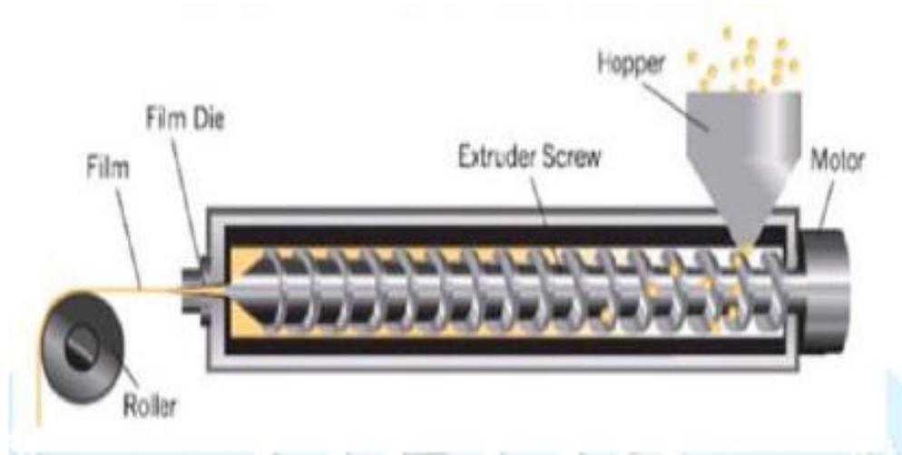
**Fig 6: Apparatus for hot melt extrusion method of preparing oral wafers.**
