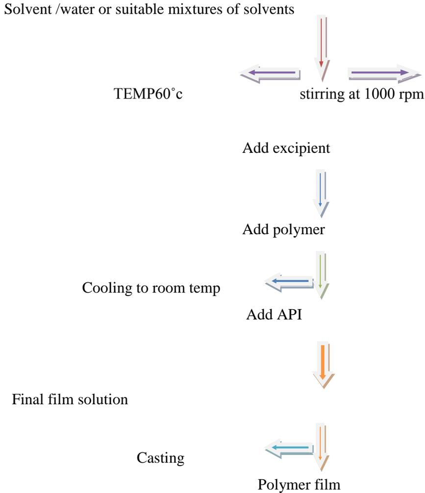
**Fig:4: Flow chart of solvent Casting method.**
