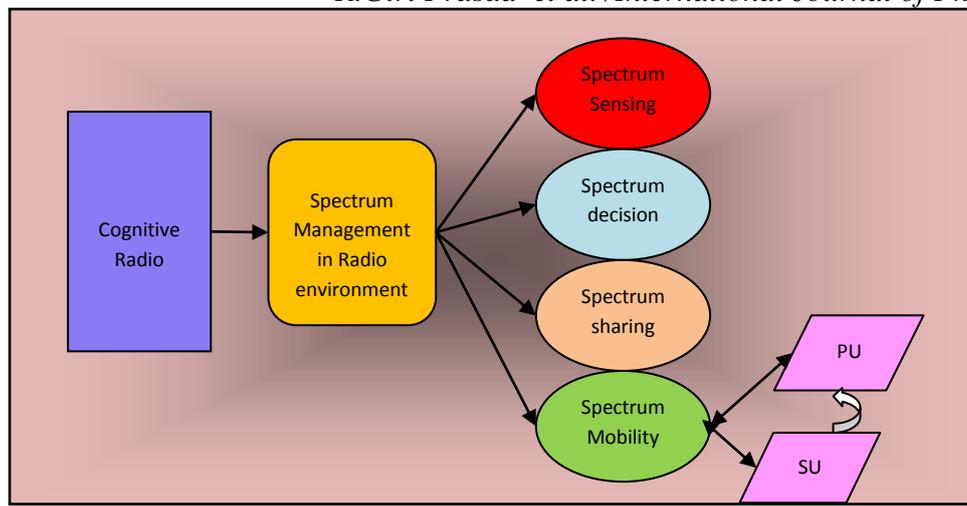
**Figure 1. Basic Architecture for Cognitive Radio Networks.**
