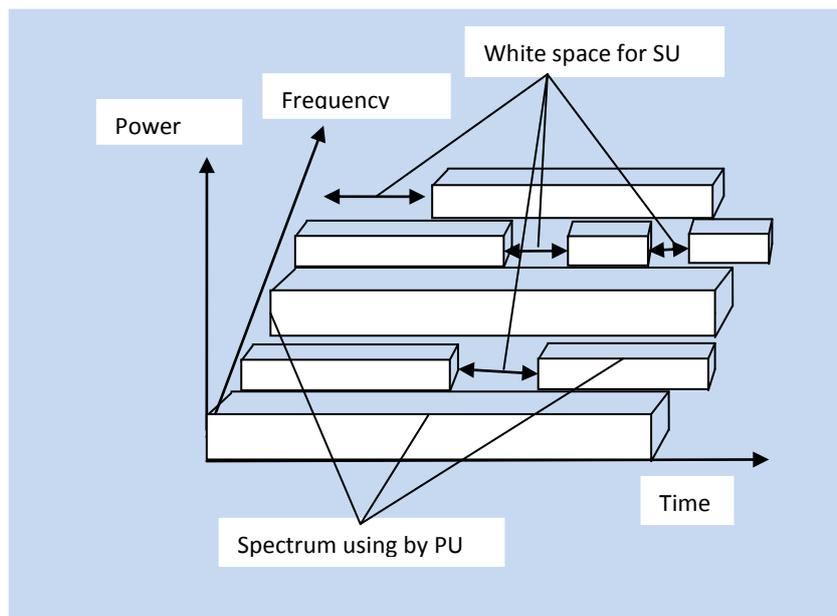
**Figure 2. Spectrum Usage by PU and SU.**
