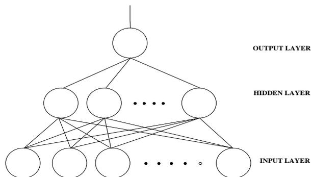
**Fig.7 A typical multi-layered feed forward network.**
