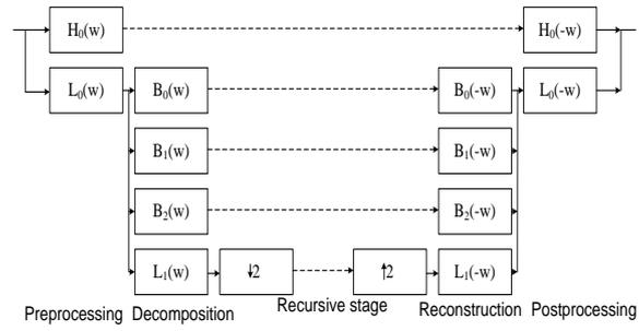
**Fig. 3 Steerable pyramid filter.**
