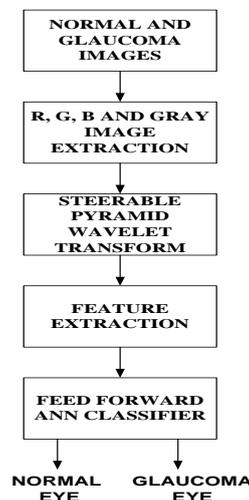
**Fig. 2 Block diagram of the proposed method.**
