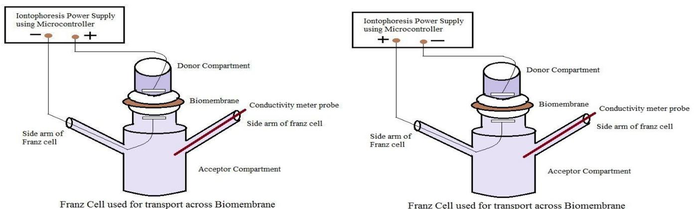
**Figure2: Iontophoretic setup that was used for iontophoretic studies of mass transport. The electrodes were connected to a Iontophoresis power supply to perform cathodal and anodal iontophoresis.**
