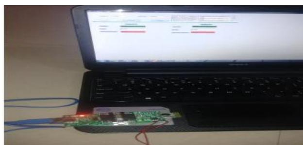
**Figure 6.3: Zigbee receiver with cloud based application.**
