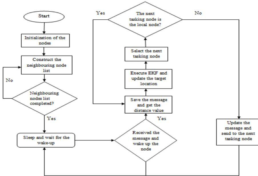
Figure 2: Flowchart of embedded application in static node.
