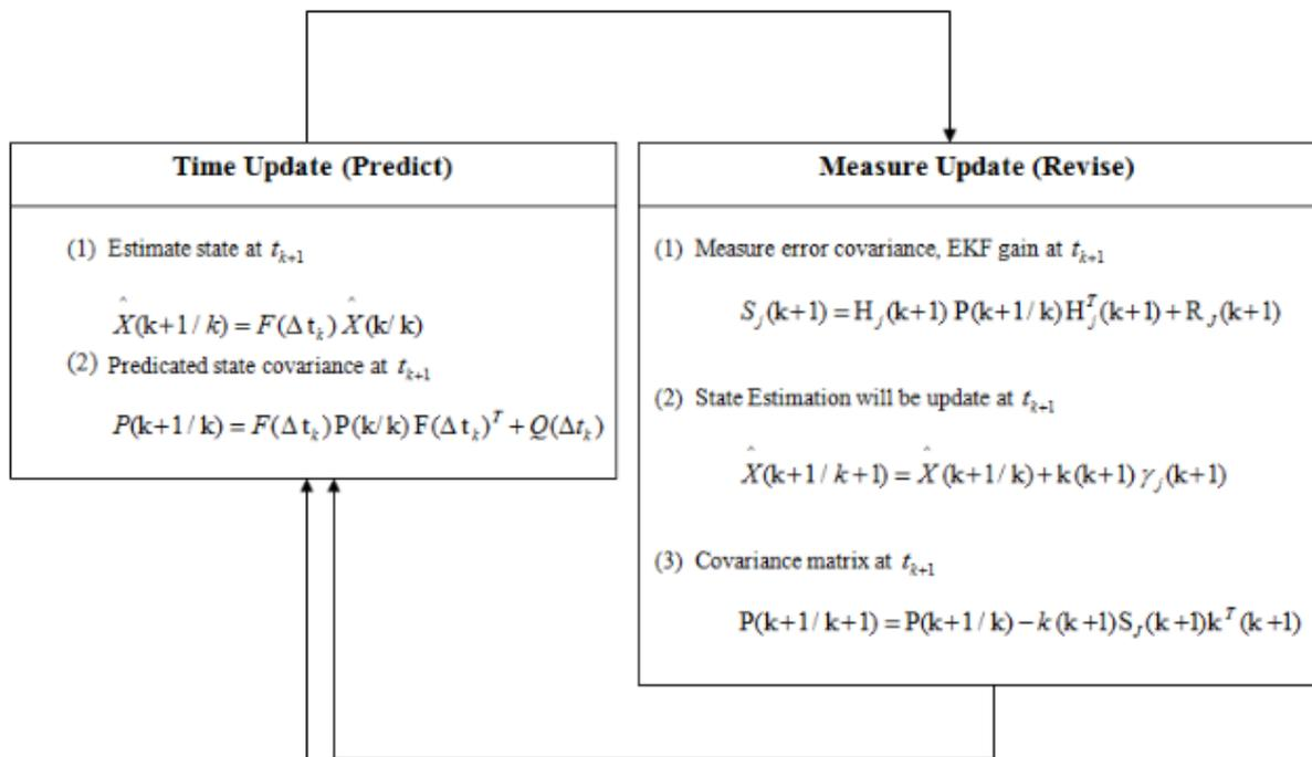
**Figure 6: Flow chart of EKF algorithm.**
