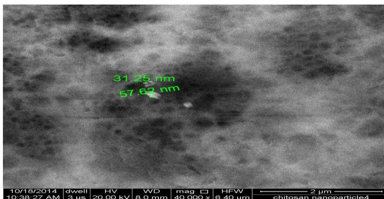
**Fig 3. SEM images of gentamicin loaded chitosan nanoparticles.**
