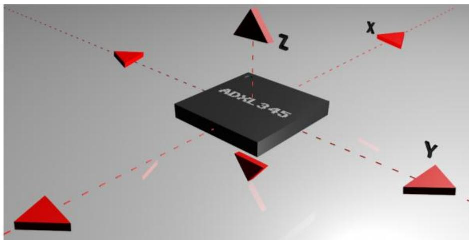
*Axes of measurement for a triple axis accelerometer*
