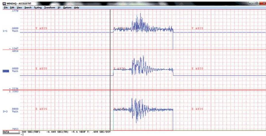
Fig. 7. Acceleration sensor output result.
