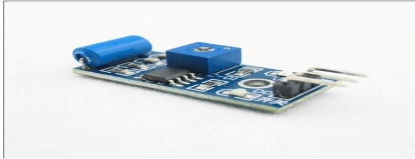
Fig. 6. Vibration sensor.
