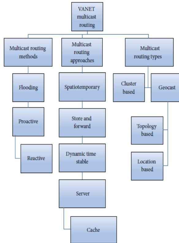
FIGURE 2: VANET multicast routing classification.
