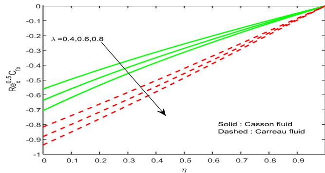
Fig.8 Effect of film thickness parameter on friction factor.
