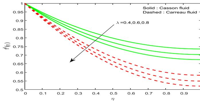
Fig.6 Effect of film thickness parameter on velocity profile.
