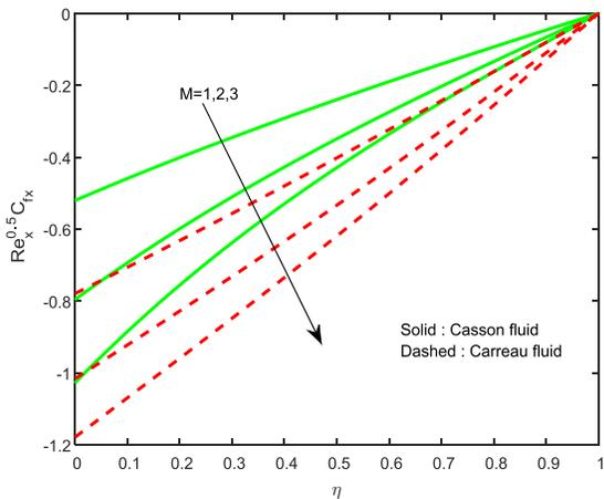
Fig.4 Magnetic field effect on friction factor.
