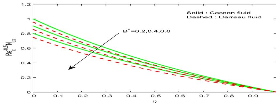
Fig.17 Effect of non-uniform heat source/sink parameter on local Nusselt number.
