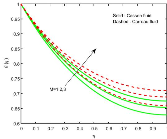
Fig.3 Magnetic field effect on temperature profiles.
