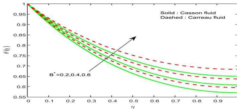
Fig.16 Effect of non-uniform heat source/sink parameter on temperature profile.
