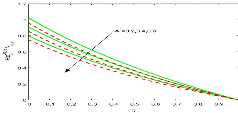
Fig.15 Effect of non-uniform heat source/sink parameter on local Nusselt number.
