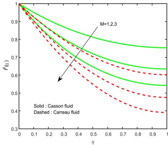
Fig.2 Magnetic field effect on velocity profiles.
