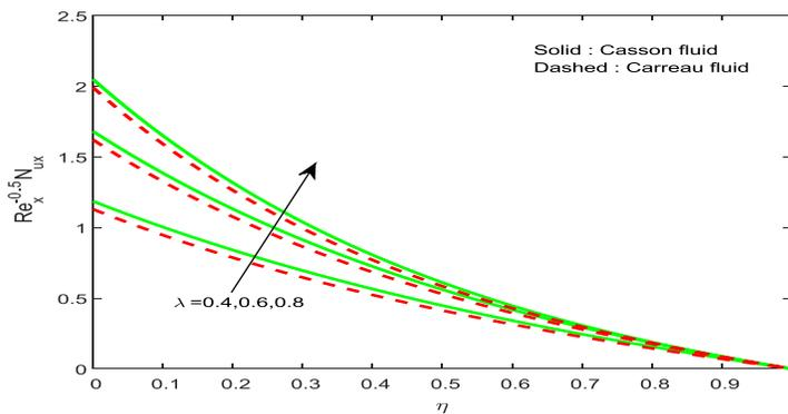
Fig.9 Effect of film thickness parameter on local Nusselt number.
