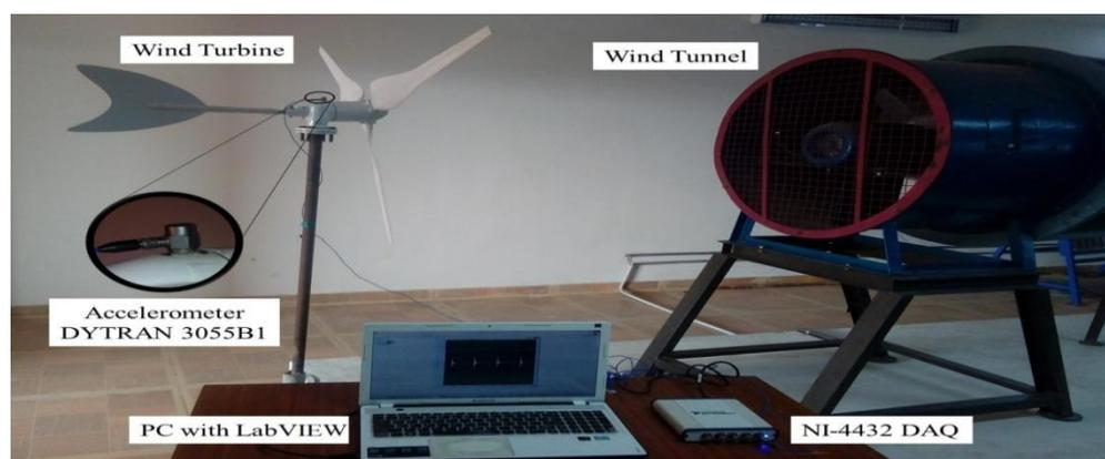
**Figure 2. Wind turbine setup.**
