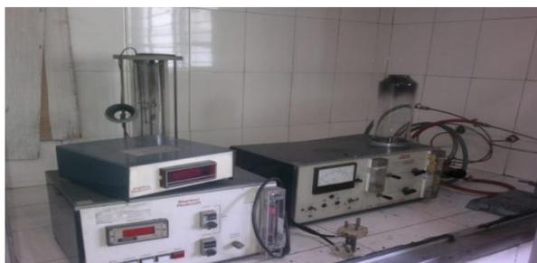
**Fig. 3. “UL 94” Horizontal Burning test apparatus (Courtesy-CPRI-Bangalore).**
