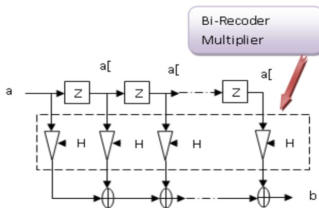
**Figure. 3 Structure of Direct Form FIR Filter.**
