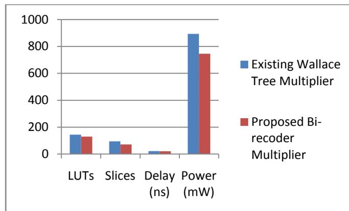
**Figure. 7 Graphical representations of Area, Delay and power.**
