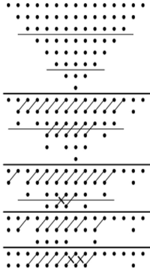
**Figure. 1 Structure of reduced complexity Wallace tree multiplier.**
