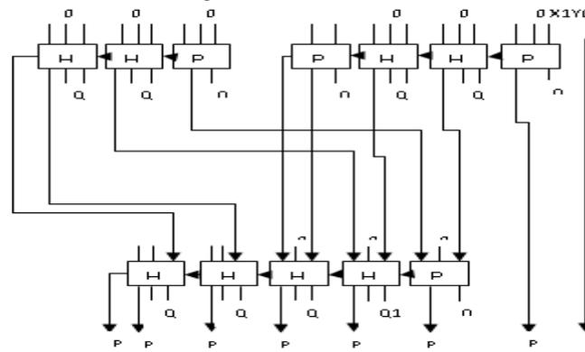
**Figure. 3 Four bit multiplier using Reversible logic gates.**
