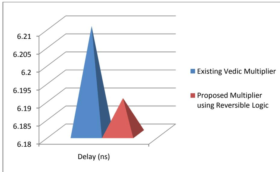
**Figure. 6 Graphical Representation of Delay.**
