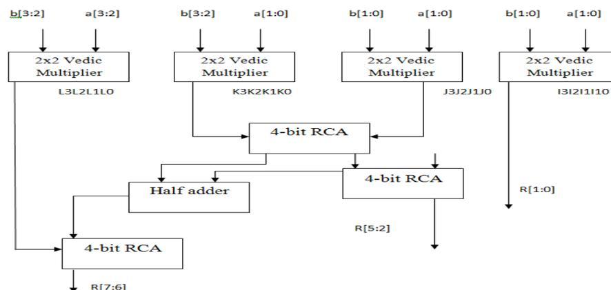
**Figure. 1 Block Diagram of 4X4 Vedic Multiplier.**
