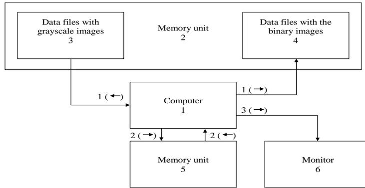
**Figure 1. Block diagram of the device that implements a method for automatically segmenting chest fluorography.**
