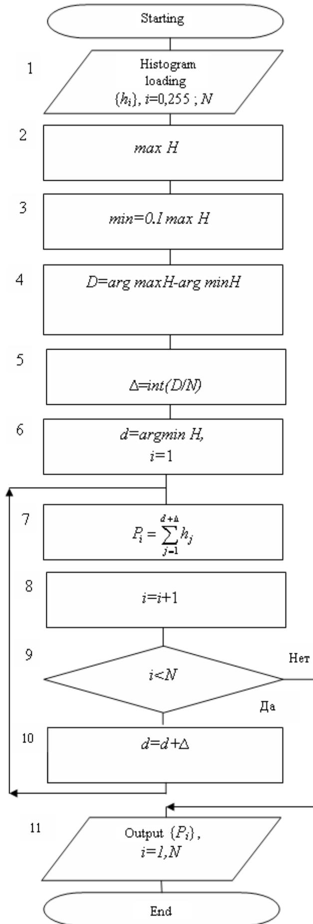
Figure 3. Scheme of the algorithm for generating the parameter vector.
