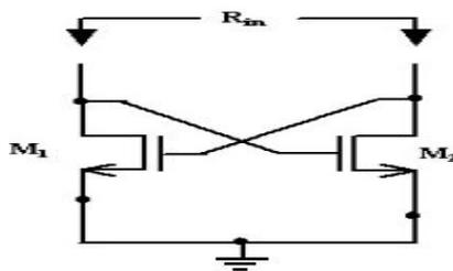
Fig. 8 NMOS cross coupled circuit.
