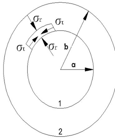
**Fig. 1. The scheme of cement stone deformation during shrinkage: 1 - filler; 2 - cement stone.**
