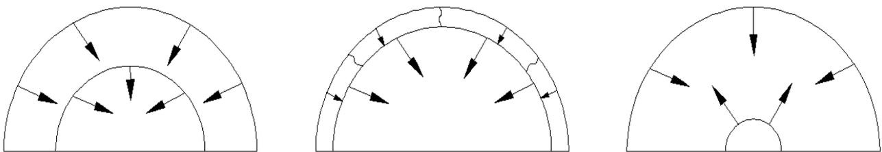
**Fig. 2. Ring shape impact concerning own shrinkage deformations of a cement stone.**
