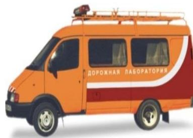
**Figure 7 –mobile laboratory of KP-514 MP type.**
