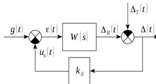
**Fig. 8. Lateral deviation control subsystem considering disturbance, which is a consequence of the nonlinearity trajectory:**
