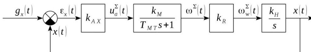
**Fig. 7. Block diagram of the longitudinal position control closed loop subsystem with a negative feedback**
