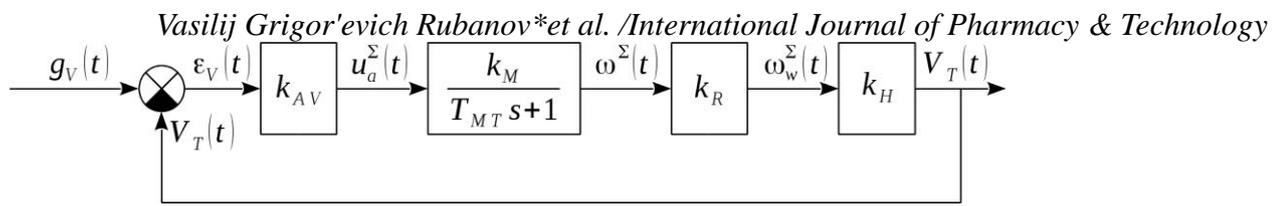
**Fig. 5. Block diagram of the longitudinal velocity control closed loop subsystem with a negative feedback.**
