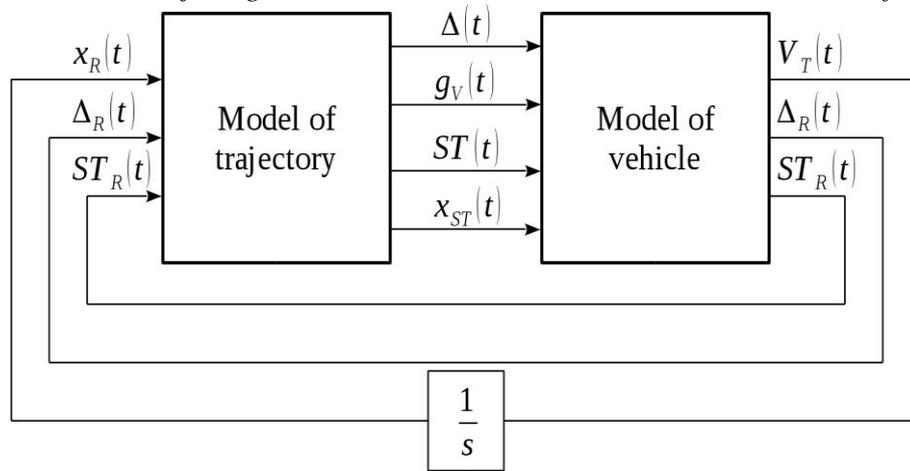
**Fig. 11. The interaction model of the trajectory and the AGV generalized model**
