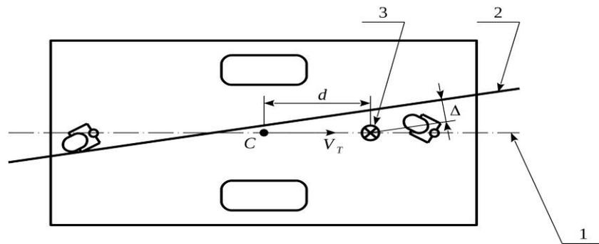
**Fig. 1. Scheme of AGV with two-wheel differential.**
