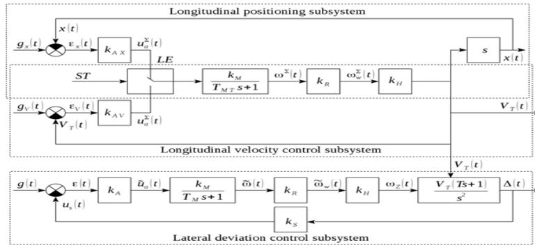
**Fig. 7. Block diagram of the generalized model of AGV motion control system.**
