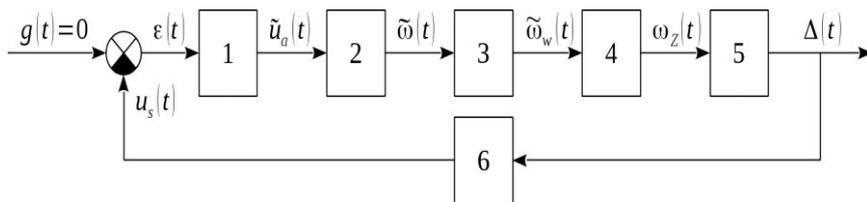
**Fig. 2. Functional diagram of the lateral deviation control subsystem:**
