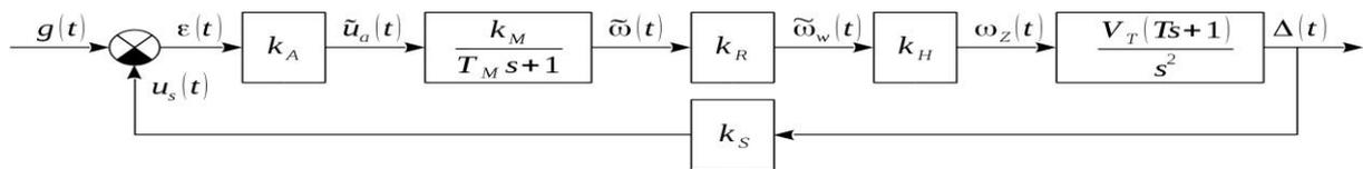
**Fig. 3. Block diagram of the lateral deviation control subsystem.**
