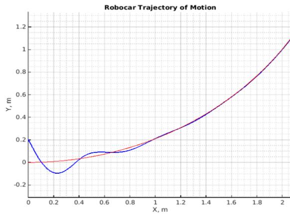
**Fig. 10. Simulation of AGV movement along the curve trajectory segment with zero initial lateral deviation.**
