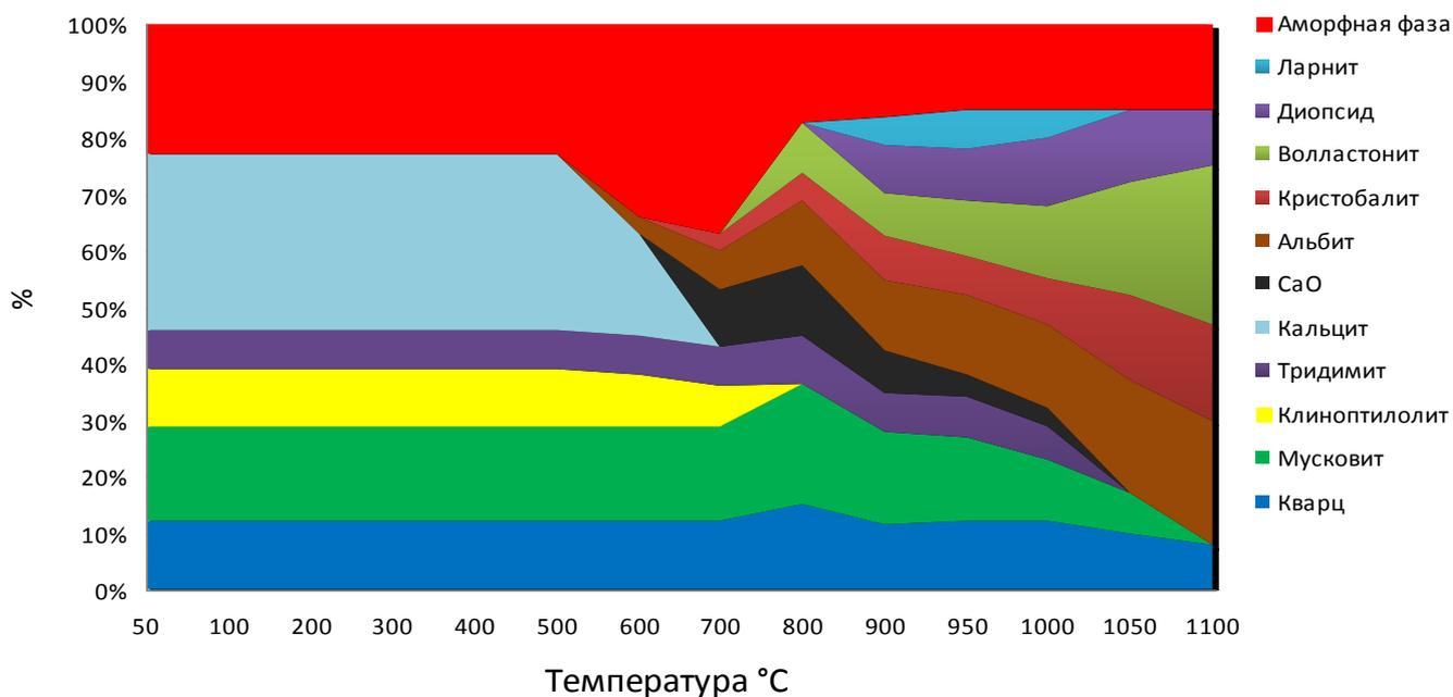
Fig. 1. Diagram of changing the phase composition of zeolite rocks Tatar-Shatrashanskoe field [10]
