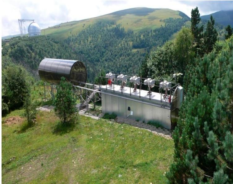
**Figure 2. Mini-Mega TORTORA optical celestial sphere monitoring system**
