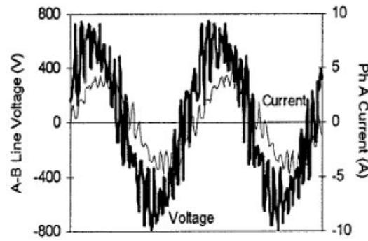
**Fig.1(b) Variable speed drive of line and load side waveform.**
