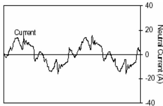
**Fig: 4. (b) Neutral current for a three phase, four wire system.**
