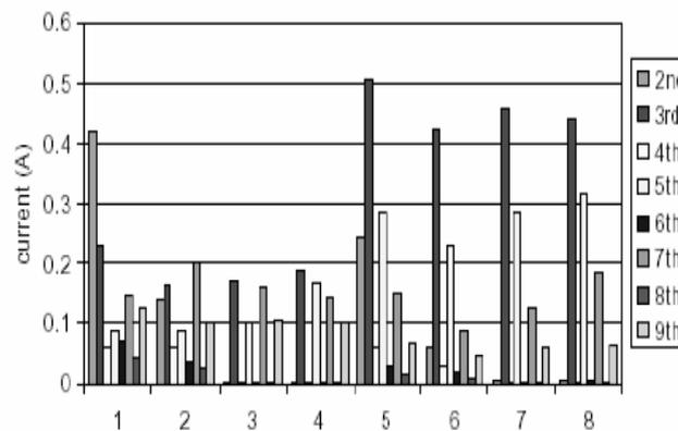
**Fig: 9 Harmonic current spectrums.**
