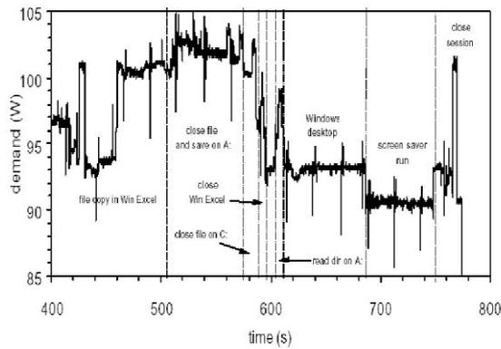
**Fig: 5 Demand diagram recorded for some typical Operations of PC.**
