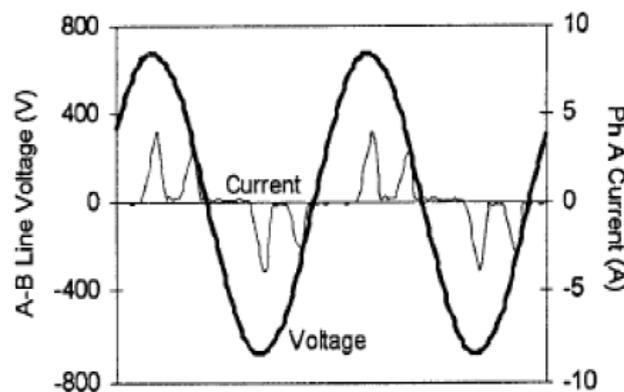
**Fig:1(a) Variable speed drive of Source and load side waveform.**
