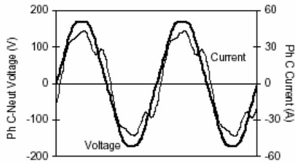
**Fig.3. (a) Phase voltage and current.**
