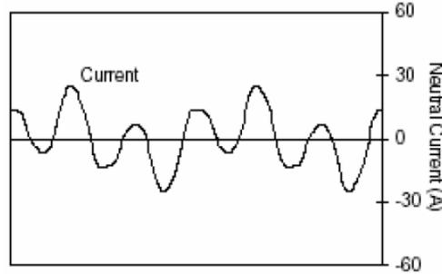
**Fig.3 (b) Neutral current for a three phase, four wire**
