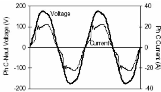
**Fig : 4. (a) Phase voltage and current**
