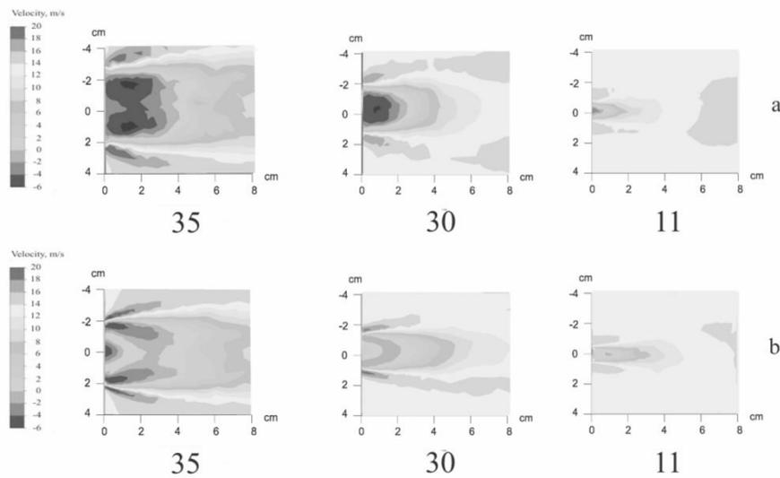
**Fig 10.** The longitudinal velocity profiles behind flameholders. a-type 1, b – type 2.
