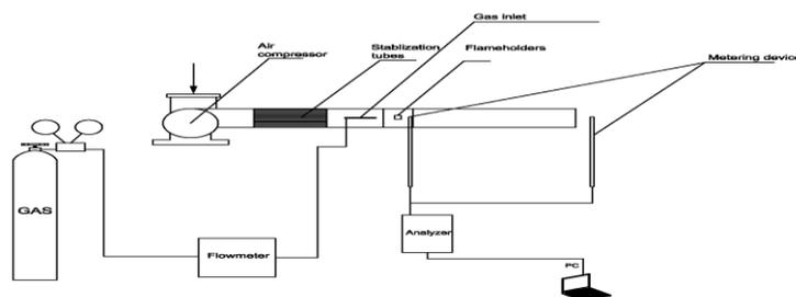
**Fig. 1.** The main diagram of the experimental setup.
