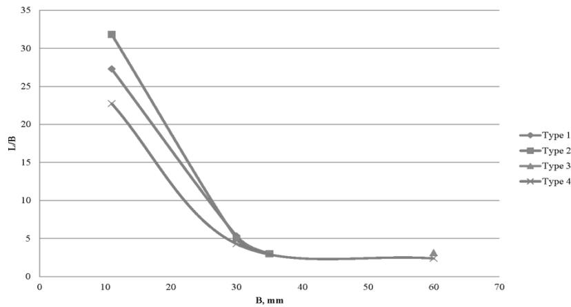
**Fig. 4.** Influence of flameholder size on the length of the flame.
