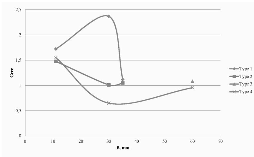
**Fig. 3.** Influence of flameholder size on the absolute air flow into the recirculation zone.
