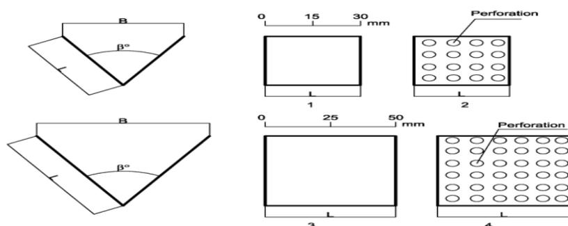
**Fig. 2.** Schematic diagrams of v-gutter flameholder: 1,2,3,4 – the types of flameholder investigated in experiment.
