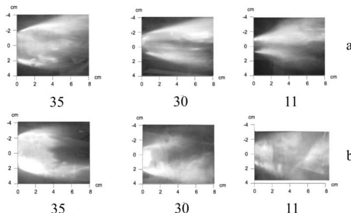
**Fig 9.** Influence of flameholder size on flame structure. a-type 1, b – type 2.
