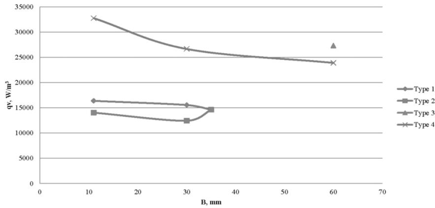
**Fig 8.** Influence of flameholder size on combustion intensity.
