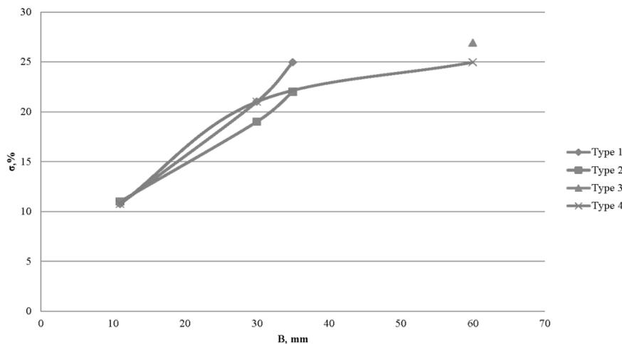
**Fig 7.** Influence of flameholder size pressure loss.
