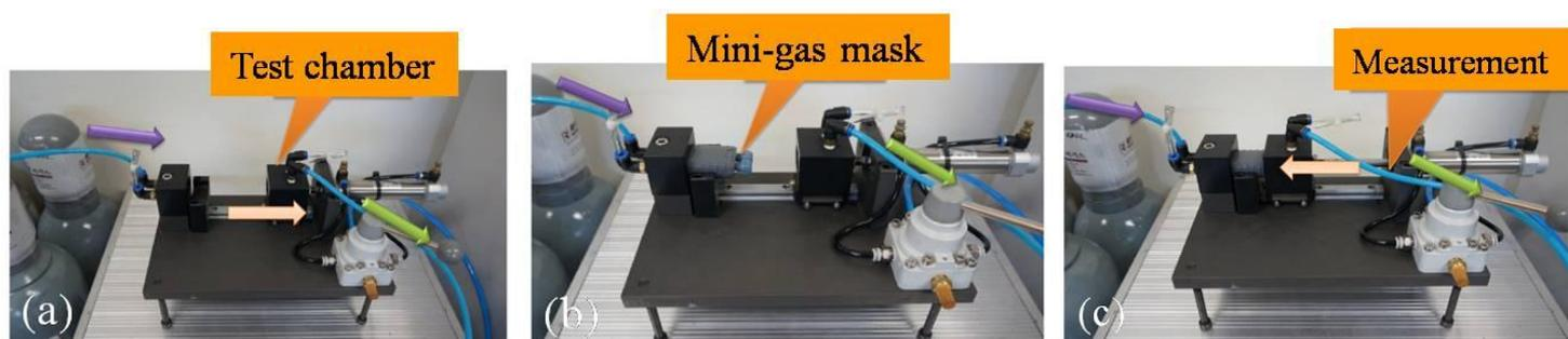
Fig. 3(a) Before setting up the fire mini-gas mask, (2) after setting up the fire mini-gas mask, and (3) measurement of CO and SO<sub>2</sub> concentration.
