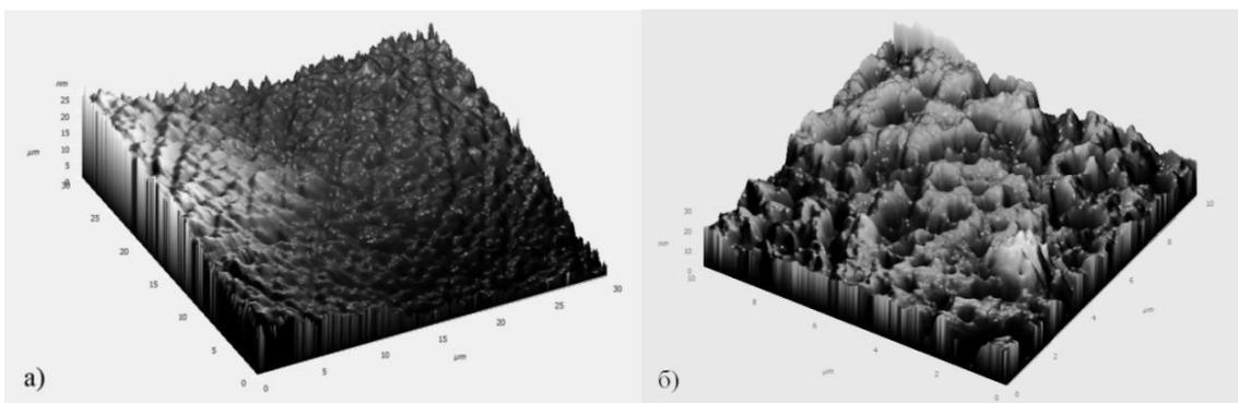
**Figure 4** – 3D AFM reconstruction of polished surface of single crystals: (a) – paratellurite, plane (110); (b) – germanium, plane (111).
