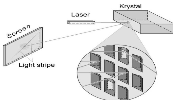
**Figure 1: Scheme explaining the appearance of laser beam reflected by the crystal.**
