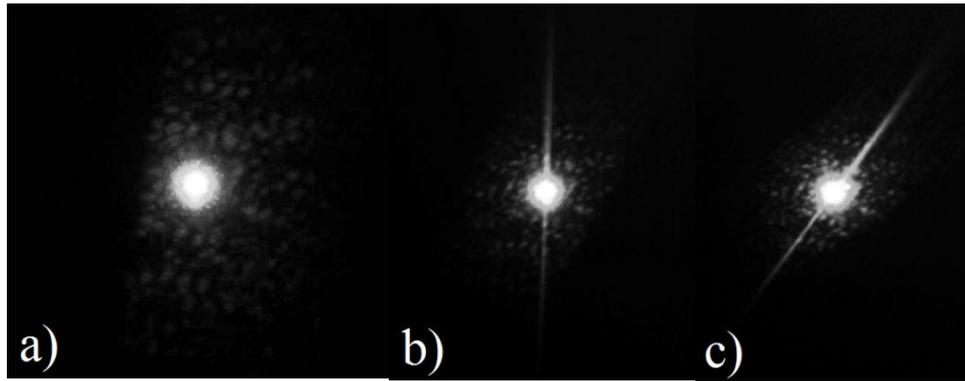
**Figure 2** – Reflection of laser light with a wavelength of 533 nm from the (001) plane of paratellurite single crystal polished to surface finish class R II with the roughness parameter  $R_a = 15$  nm (a), and from the plane (110) after rotation of the crystal. The observations were made at a distance of 7 m (b, c). The bands of reflection are elongated along the straight line  $[\bar{1}10]$ .
