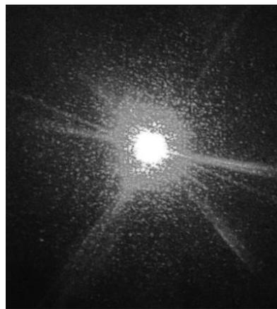
**Figure 3** – Laser light reflection from the (111) plane of germanium polished to surface finish class R II with roughness parameter  $R_a = 22$  nm as observed at a distance of 7 m. The reflection bands are elongated along three straight lines  $[1\bar{1}\bar{1}]$ ,  $[\bar{1}1\bar{1}]$ ,  $[\bar{1}\bar{1}1]$ .
