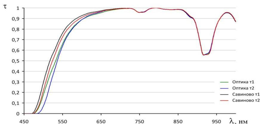
**Fig. (3)** – Oil transmission spectra of T-1500 type (s/s "Optics" and "Savinovo" KES).
