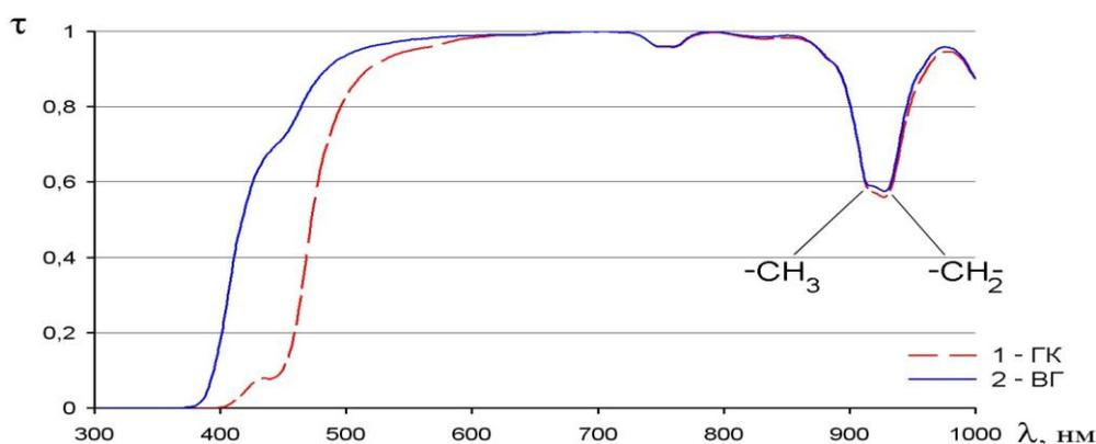
**Fig. (1)** – VG and GK oil transmission spectra.
