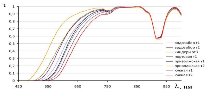
**Fig. (5)** – TKp oil transmission spectra, obtained from KES transformers.
