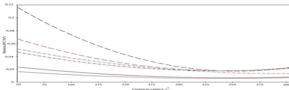
**Fig. (1)** – The dependence of dynamic viscosity of coal-water fuel samples and the compositions on its basis on shear rate at various temperatures
