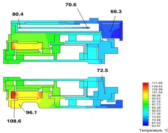
**Figure 5** – Imitation of work in space without solar radiation ( $T_{env.} = -269^{\circ}C$ ,  $Q_s = 0 \text{ W/m}^2$ ).
