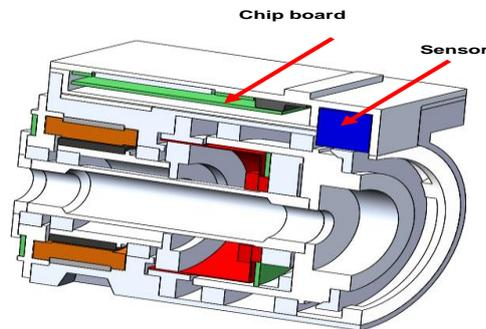
**Figure-2** – Cross-section of a joint of the RAT.
