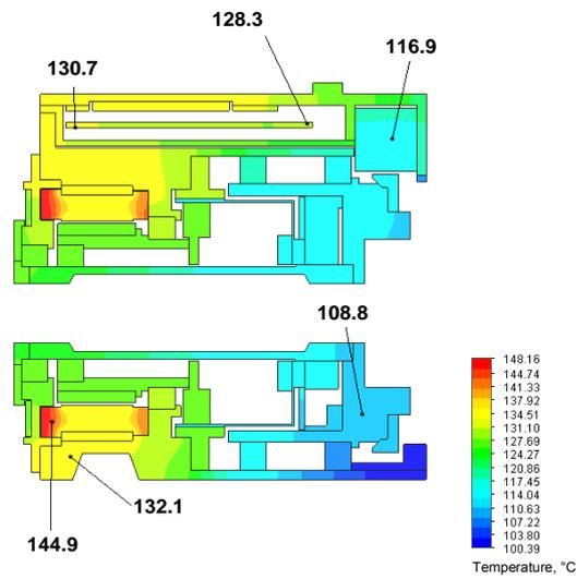
**Figure 4** – Imitation of work in space taking into account solar radiation ( $T_{env.} = -269^{\circ}C$ ,  $Q_s = 1422 \text{ W/m}^2$ )
