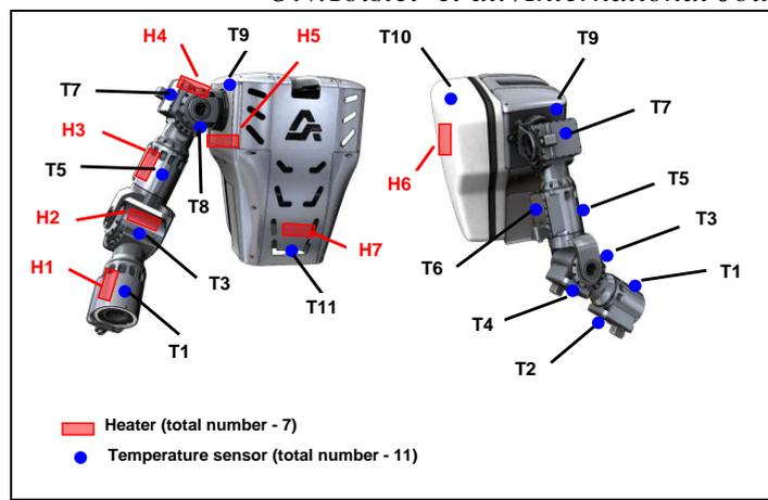
**Figure 1** – Position of temperature sensors and heaters on the RAT.
