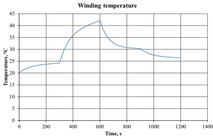
Figure 7 – Imitation of work in vacuum chamber ( $T_{env.} = 20\text{ °C}$ ). Dynamic calculation by a cyclogram: 4,8 W – 300 s, 24 W – 300 s, 4,8 W – 300 s, 0 W – 300 s, , initial temperature of the joint 20 °C.
