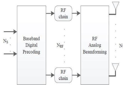
**Fig.3. Hybrid structure for Beam Forming of millimetre wave transmission.**
