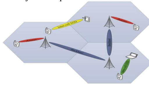
**Fig.1. millimetre wave 5G cellular mobile network with Device 2 Device (D2D) communication.**
