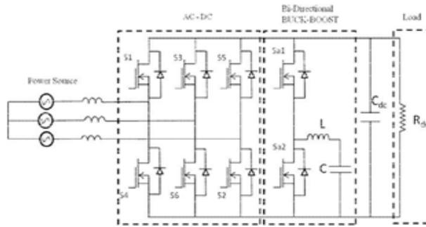
**Fig. 1. Proposed Active Rectifier**
