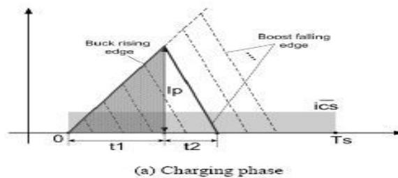
**Fig. 2. Boost mode during charging phase.**
