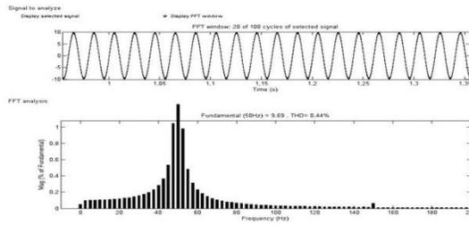
**Fig. 13. Harmonic analysis for closed loop.**
