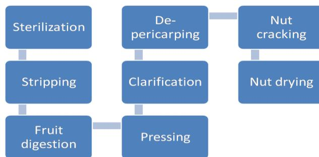
**Figure 5: Oil extraction process.**
