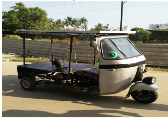
**Fig 2. Proposed model of Hybrid Auto Rickshaw.**
