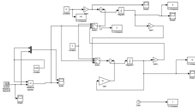
**Figure 5: The mathematical modelling of the boost converter**
