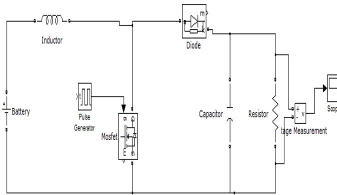
**Figure 4: boost converter circuit.**
