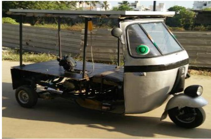
**Fig 11: Prototype of hybrid electric vehicle.**
