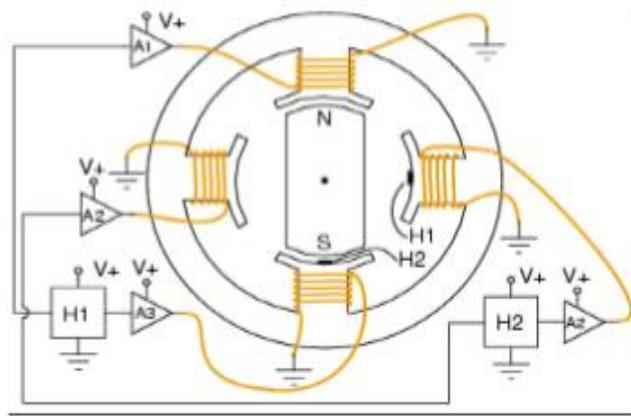
**Fig 7: Diagram of BLDC motor**
