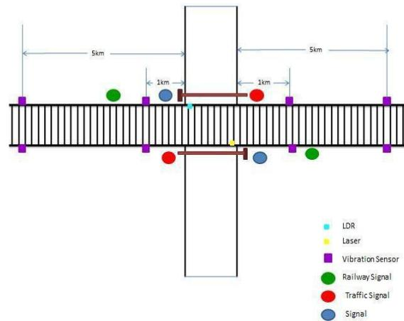
**Fig. 1 demonstrates the stream diagram of the entryway shutting operation.**
