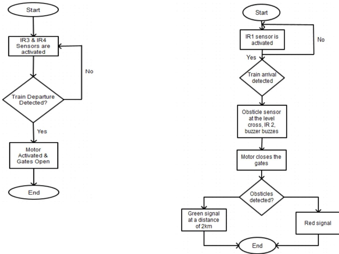
**Fig. 2 Flow chats for opening gates (and) Fig.3 Flow chart for closing gates.**
