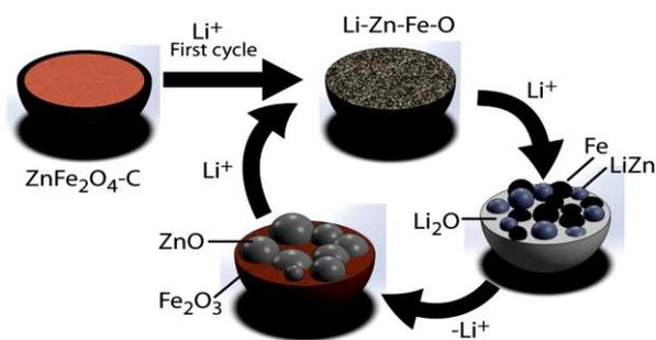
**Fig. 2 lithiation–delithiation main reactions, which occurs in zinc ferrite NPs (ZnxFe<sub>3-x</sub>O<sub>4</sub>).**
