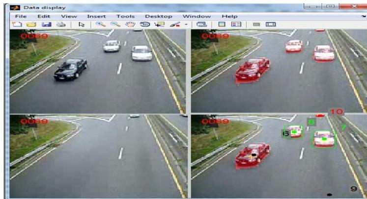
**Figure 2. Moving cars detection and tracking from static video.**
