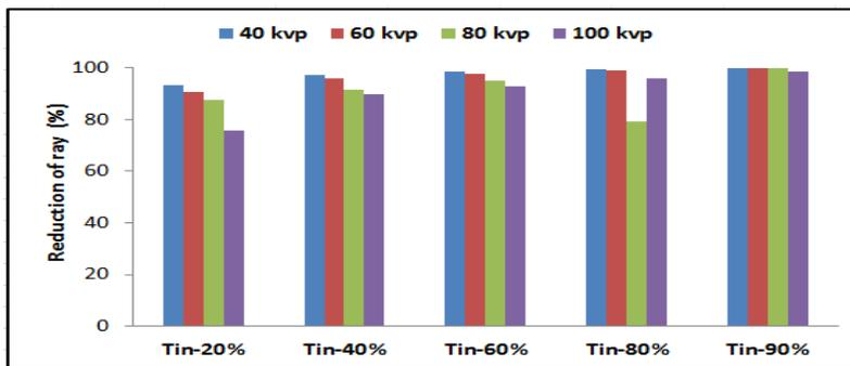
Figure-2. The mean percentage of X-ray attenuation by different Nano size combinations of tin dioxide in voltages 100, 80, 60 and 40 kVp.
