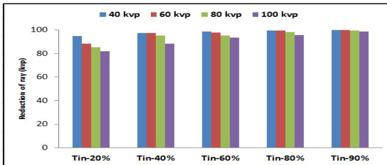
Figure-3. The mean percentage of X-ray attenuation by different Micro size combinations of tin dioxide in voltages 100, 80, 60 and 40 kVp.
