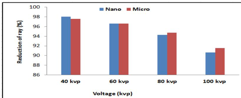
Figure-4. The mean percentage of X-ray attenuation by different Nano and Micro size combinations of tin dioxide in voltages 100, 80, 60 and 40 kVp.
