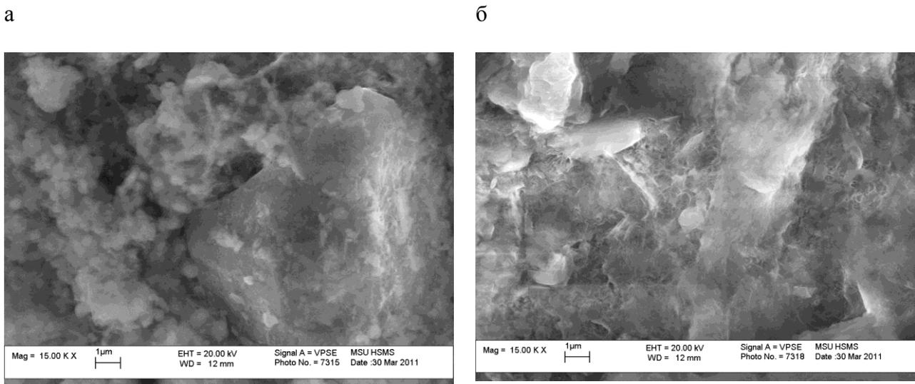
Fig. 2. The microstructure of samples based on loam containing 10 wt. % of lime, SEM:
