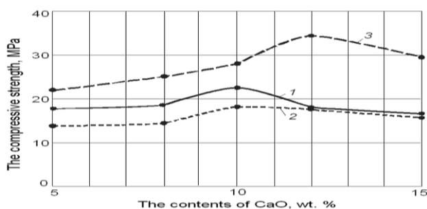
Fig. 1. Maximum compressive strength of the samples according to the content of lime:
