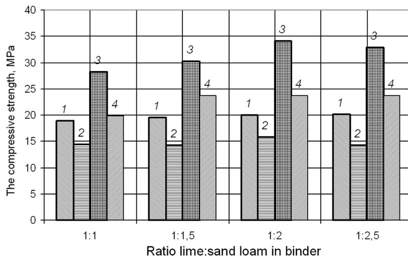
Fig. 3. The maximum compressive strength of the samples based on LSCB depending on a binder composition:
