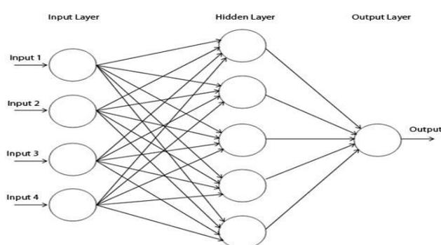
Neural Network Architecture characterizes its structure including number of hidden layers, number of hidden nodes, number of output nodes and activation function
