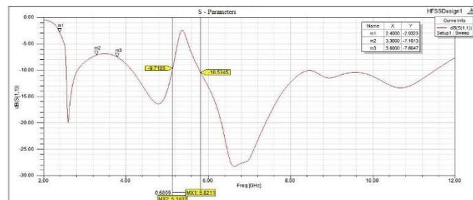
**Fig.2  $S_{11}$  parameters of MIMO antenna.**
