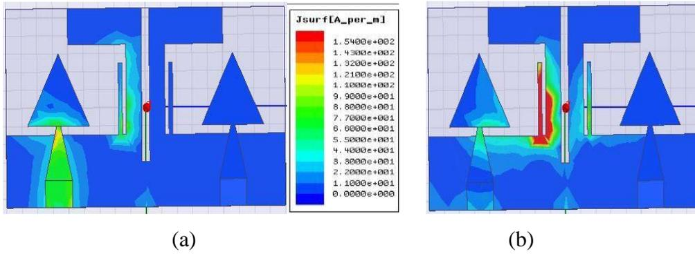
**Fig.4 Surface Current distribution at (a) 4 GHZ (b) 5.4 GHZ.**
