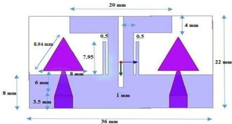
**Fig.1 Geometry of antenna (dark gray: antenna patch, light gray: ground).**
