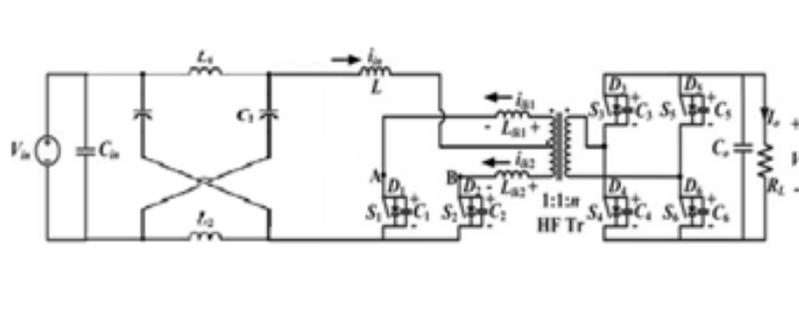
**Fig. 1. Circuit diagram of Z- source push pull DC-DC converter.**
