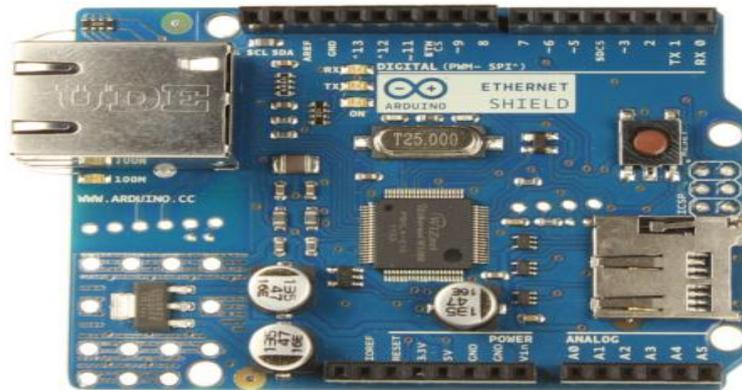
**Figure.2 Arduino Ethernet Shield.**
