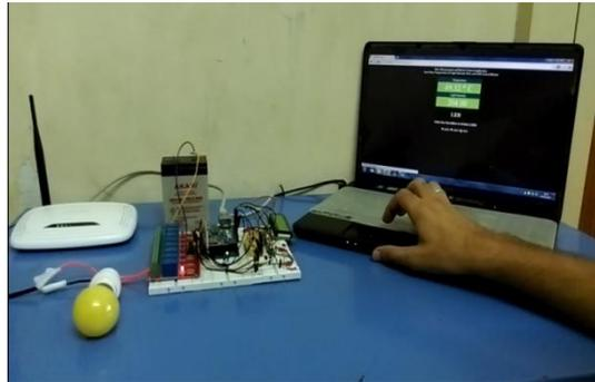
Figure.9 Appliances in OFF State via Web Control.
