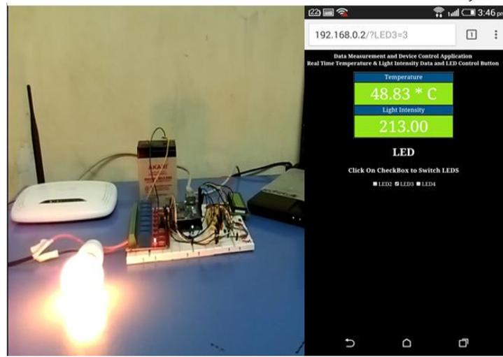
**Figure.12 Appliances in ON State via Mobile Control.**
