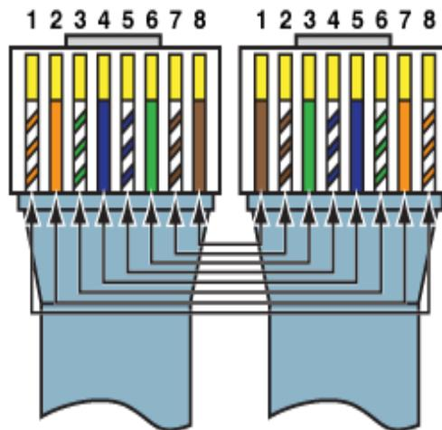
**Figure.4 RJ45 Connector.**
