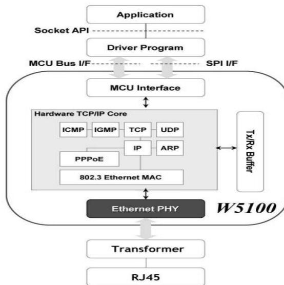
Figure.1 Block Diagram of Wiznet W5100.
