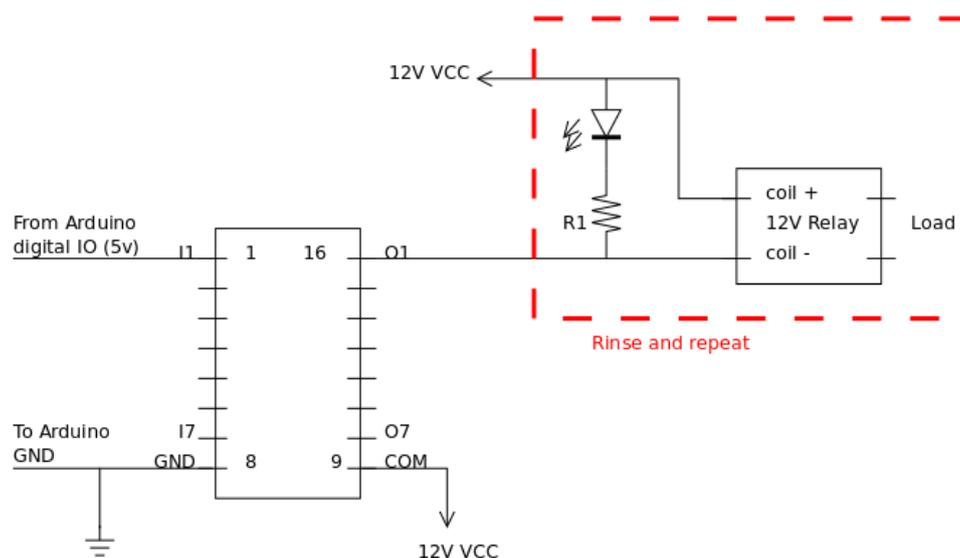
Figure.5 Relay Connection through MCU and Driver.
