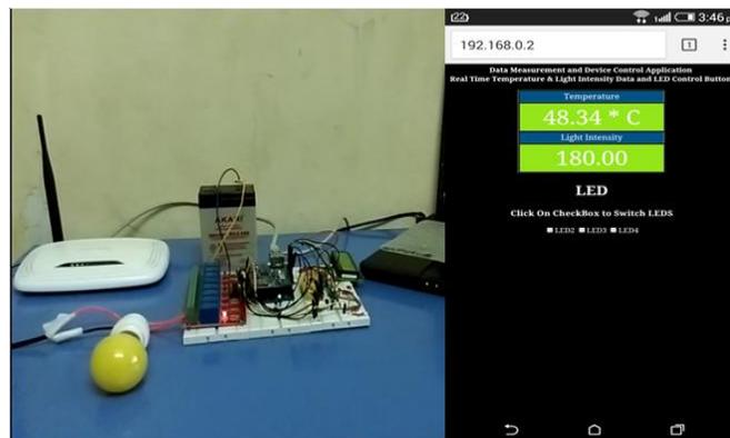
Figure.11 Appliances in OFF State via Mobile Control.
