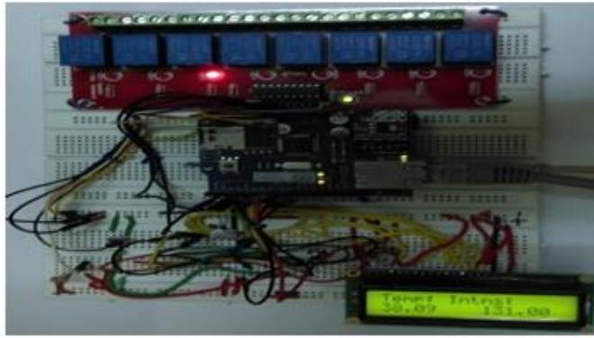
Figure.8 Ethernet Connect with MCU, LCD, Sensors, Relay.
