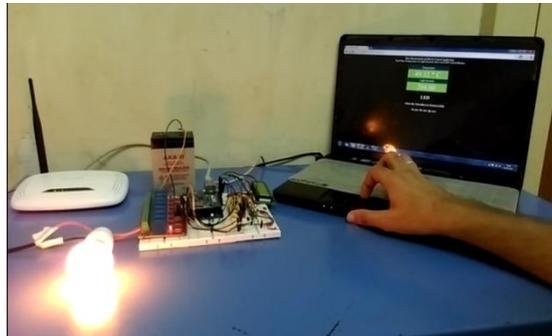
Figure.10 Appliances in ON State via Web Control.
