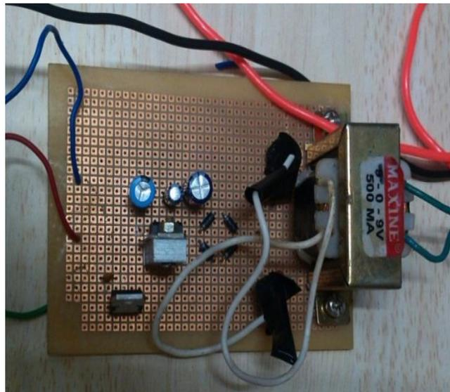
Figure.7. Regulated power supply.
