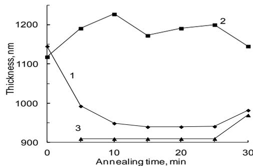
**Fig. 5.** The dependencies of coating thickness on the annealing time: 1 - coating thickness according to ellipsometry data, 2 - coating thickness according to electron microscopy, 3 - the thickness of the sintered portion according to microscopy data.
