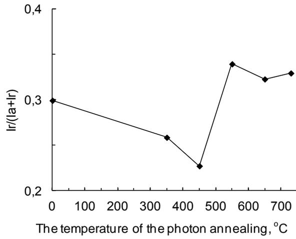
**Fig. 16. The dependence of the peak intensity ratio (110) to the sum of anatase (101) and rutile (110)  $I_r/(I_a+I_r)$  on temperature.**
