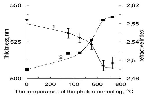
**Fig. 14. Photon annealing temperature dependence on the thickness of coating (1) and the refraction index of the base layer (2) defined by ellipsometric method.**
