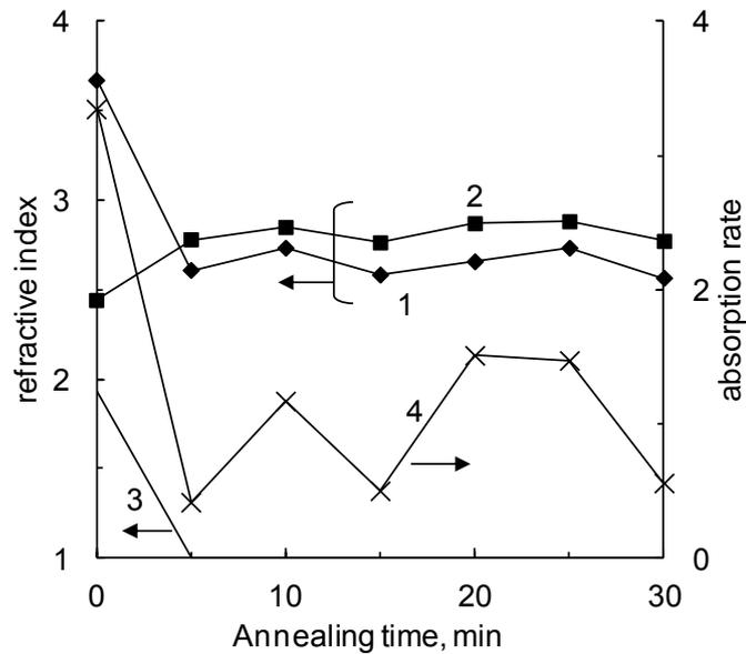
**Fig. 3. Dependencies of refractive (1-3) and absorption (4) index of layers on the annealing period; 1, 4 - contact layer, 2 - base layer, 3 - roughened layer.**
