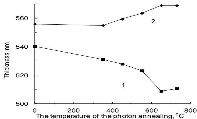
**Fig. 18. The dependencies of coating thickness on the annealing temperature: 1 - coating thickness according to ellipsometry data, 2 - coating thickness according to electron microscopy data.**
