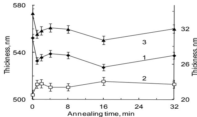
**Fig. 8.** The dependencies on the duration of the coating layer thickness annealing (the first series of samples): 1 - base layer, 2 - rough layer, 3 - coating thickness.
