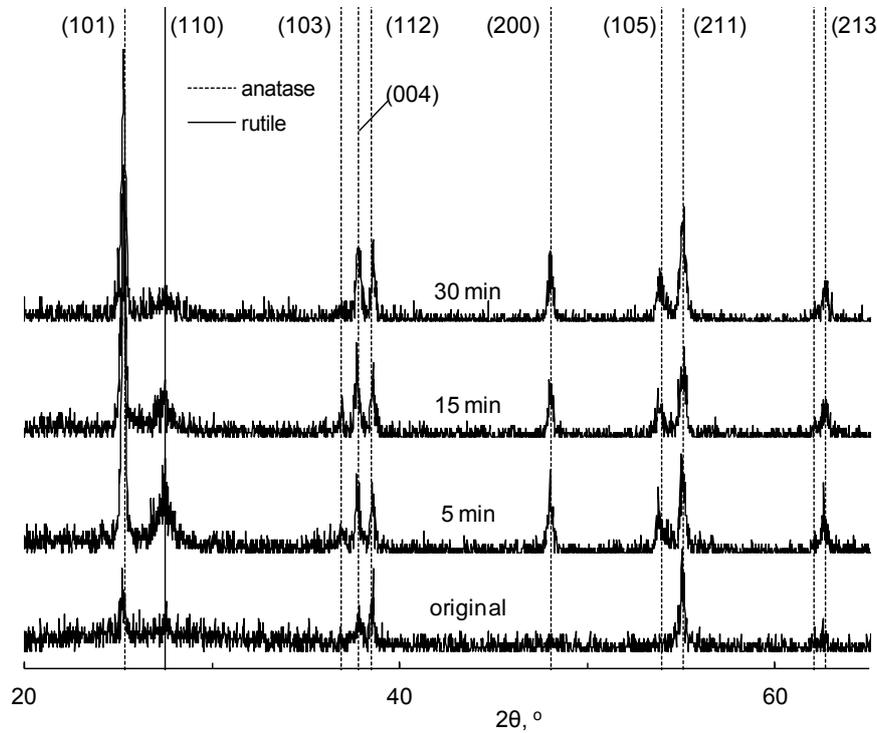
**Fig. 6. Diffraction patterns of coatings depending on the duration of photon annealing for the third series of samples.**
