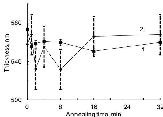
**Fig. 13. The comparison of TiOx coating thickness obtained by ellipsometry (1) and microscopy (2) for the first series of samples.**
