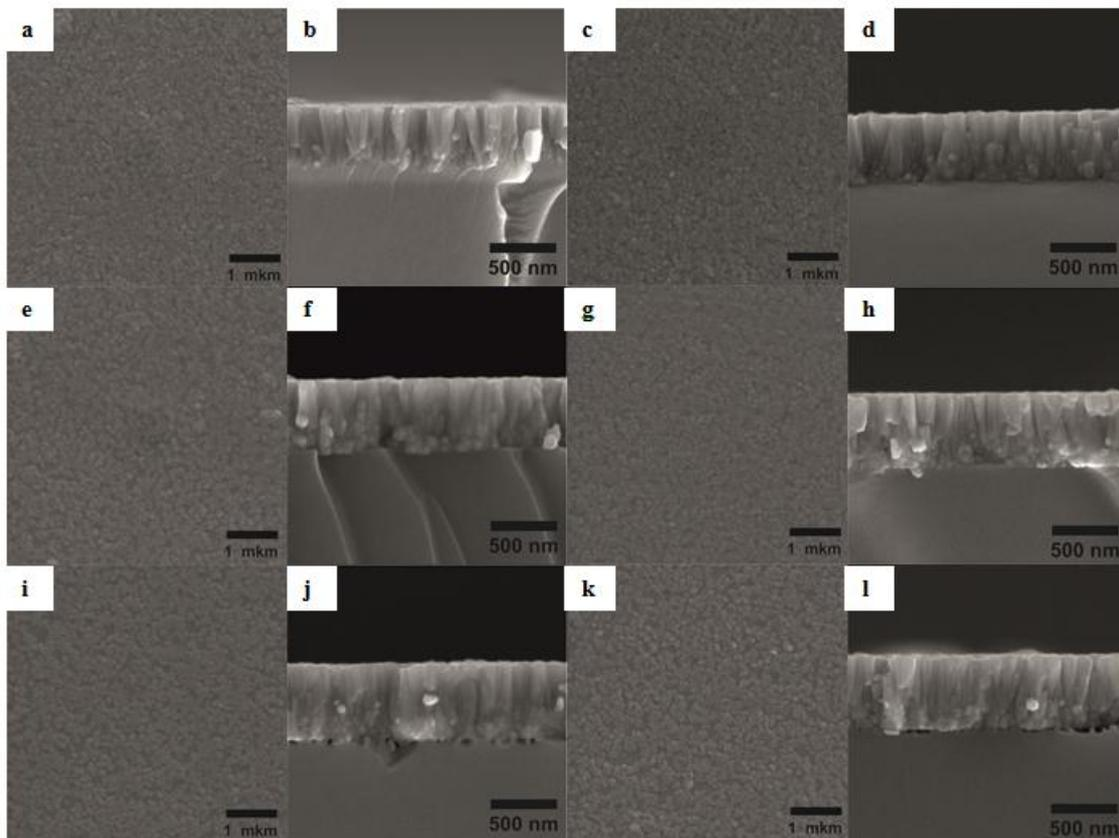
**Fig. 17. The fracture patterns and the surface of TiO<sub>2</sub> thin films, photon annealing for 4 minutes at the temperature of: a, b - without annealing; c,d –350°C; e,f – 450°C; g,h – 550°C; i,j –650°C; k,l – 730°C.**
