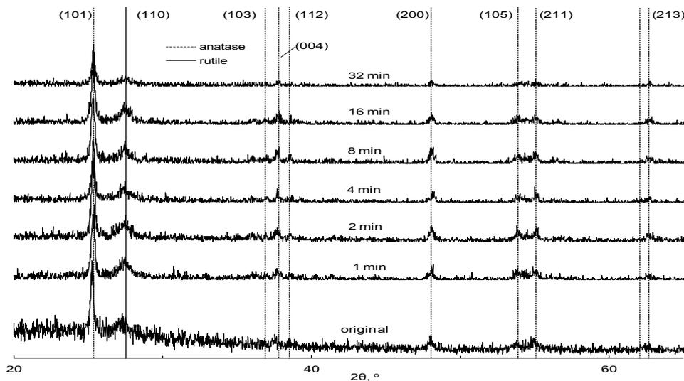
**Fig. 9.** Diffraction patterns of coatings depending on the duration of photon annealing for the first series of samples.
