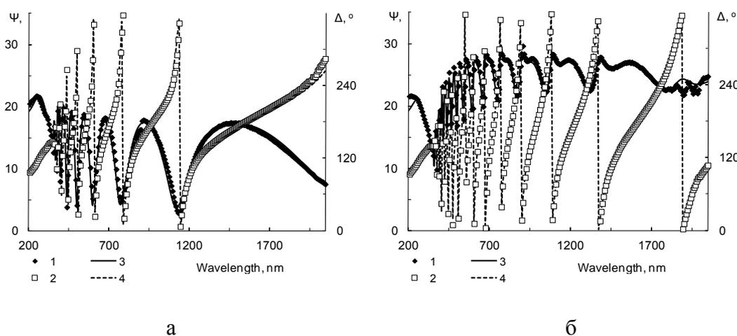
**Fig. 1. The spectral dependences of measured (1, 2) and model (3, 4) ellipsometric angles ([PSI] and [DELTA]) for the samples deposited at 20 vol. % of O2 (a) and 10 vol. % of O2 (b) 1, 3 - [PSI], 2, 4 - [DELTA].**
