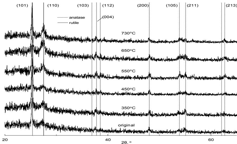
**Fig. 15. Diffraction patterns of coatings depending on the duration of photon annealing for the first series of samples.**
