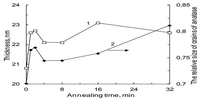
**Fig. 10. The dependencies on the period of annealing concerning the relative volume of anatase grains (1) and the height of the roughness layer (2).**
