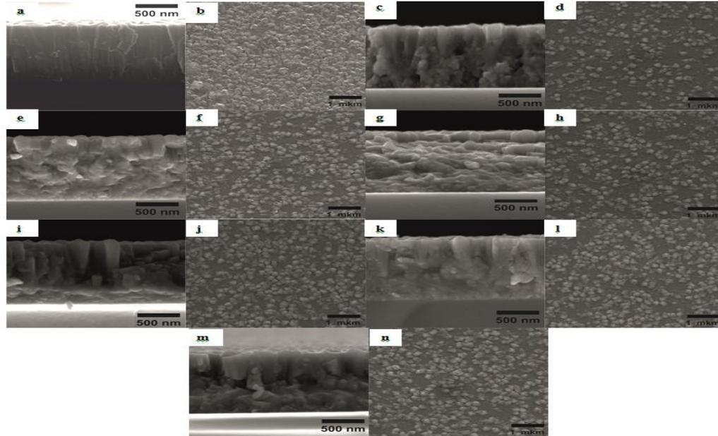
**Fig. 4.** The fracture patterns (a, c, e, g, i, k, m) and the surface (b, d, f, h, j, l, n) of  $\text{TiO}_x$  coatings depending on the time of photon annealing for the third series of samples: a, b – without annealing; c, d – 5 min; e, f – 10 min; g, h – 15 min; i, j – 20 min; k, l – 25 min; m, n – 30 min.
