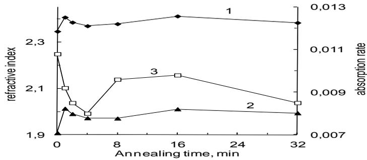
**Fig. 12. The dependence of the refraction (1,2) and absorption (3) index in coating layers on the annealing duration: 1, 3 - base layer, 2 - roughened layer.**
