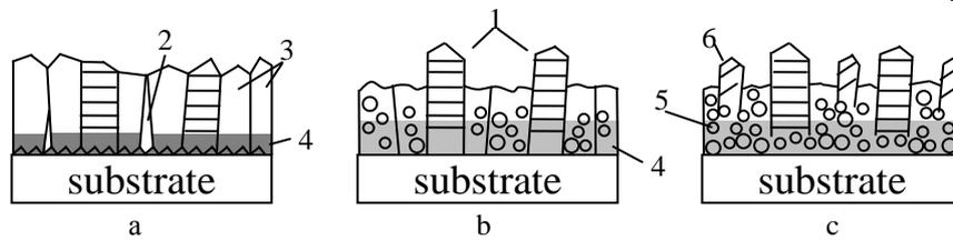
**Fig. 7.** Approximate scheme of the structure change in terms of photon annealing at 500 °C for TiO<sub>x</sub> coatings with an excessive content of Ti in the contact layer: a - original coating, b - short annealing, c - prolonged annealing, 1 - grain, polished by low-energy facets, 2 - pore, 3 - defective grains, 4 - the layer with the excess of Ti, 5 - sintered areas 6 - the grains grown from sintered portions.
