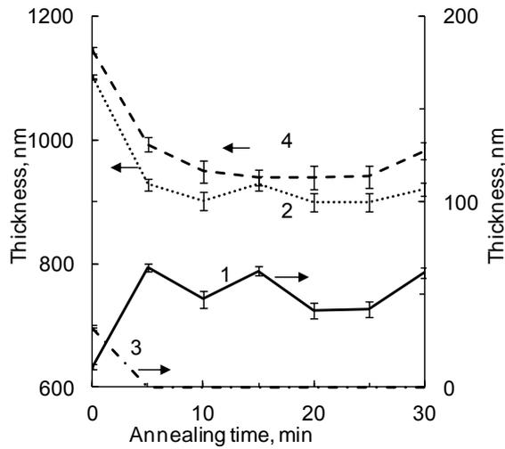
**Fig. 2. Dependencies on the duration of annealing for the thickness of coating layers (the third series of samples): 1 - contact layer, 2 - base layer 3 - rough layer 4 - coating thickness.**
