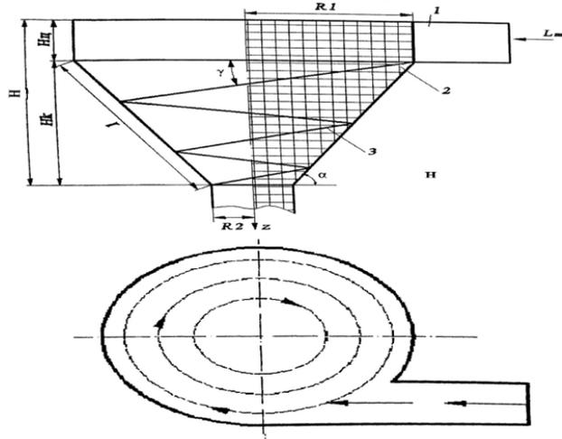
**Fig. 1. Centrifugal classifier for the separation of raw cement sludge: 1 - inlet branch, 2 - filtering screen; 3 - directing spiral vane.**
