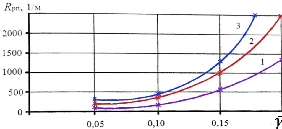
Fig. 2. The dependence of filtration resistance from partition wall I ratio on its living section ratio and filtration speed: 1 —  $v_{sp} = 0,002$  m/s; 2—  $v_{sp} = 0,0035$  m/s; 3—  $v_{sp} = 0,0045$  m/s.
